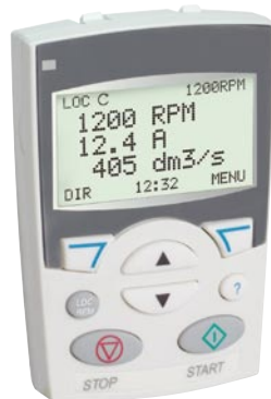
Assistant control panel
